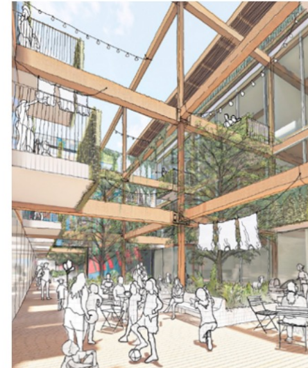
A central courtyard is carved out of the center of the block to provide light and air to residential units. The timber structure is maintained as a spatial remnant of the historic warehouse use.
