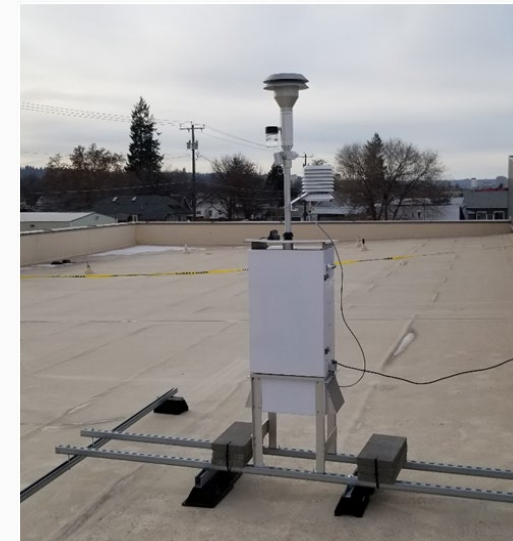
Ecology's custom-built SensWA PM 2.5 sensor
