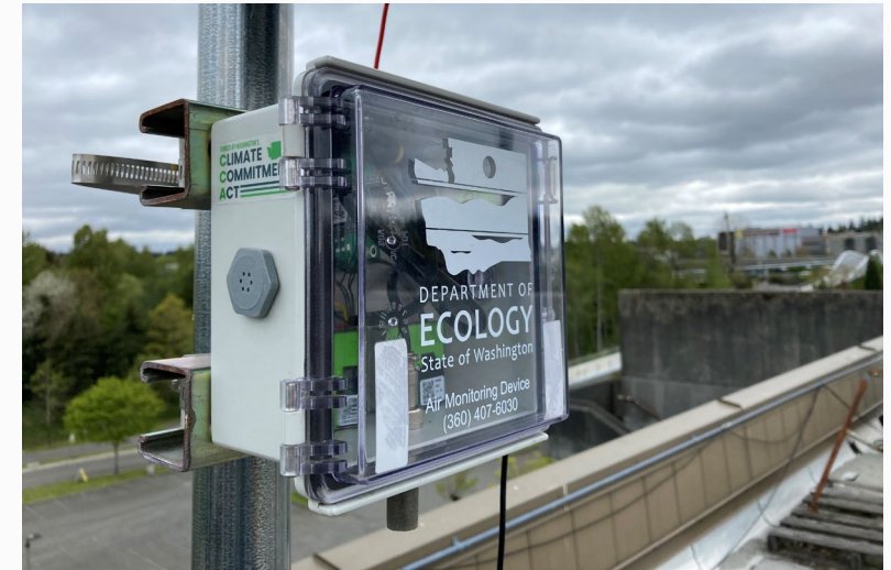
Ecology's custom-built SensWA PM 2.5 sensor
