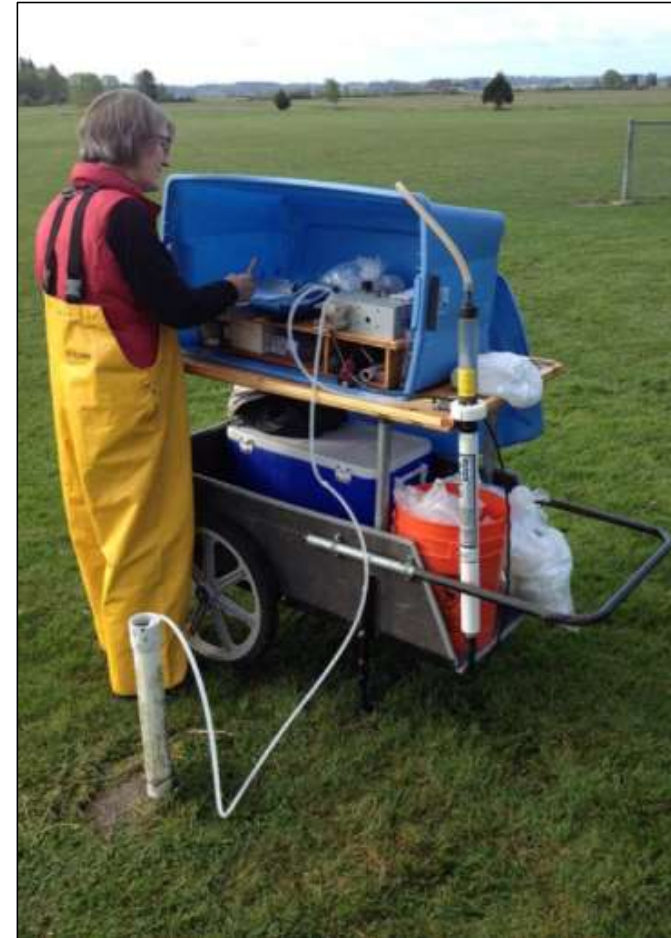
Ecology Hydrogeologist sampling a groundwater monitoring well.
