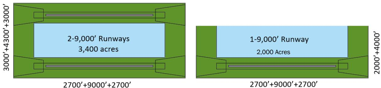
These layouts were then used to analyze the area surrounding the study area airports to determine whether sufficient space exists to accommodate commercial service and cargo needs with limited impacts to existing developed areas.
