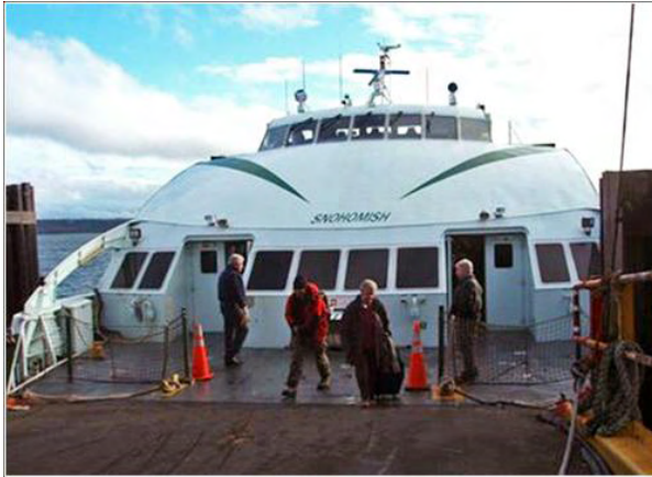
Bow loading vessels allow rapid boarding and debarking.
