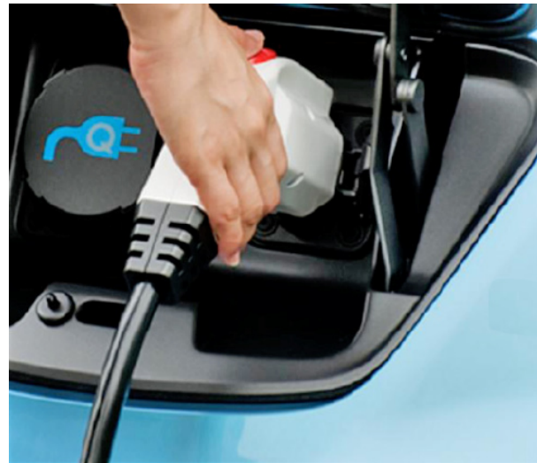
Figure 2. The J1772 connector will be the standard charging plug for all new electric vehicles. Photo courtesy of Nissan.
